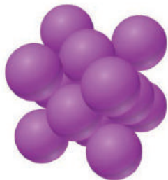
Figure 12.30 Cubic closest packing of argon (face-centered cubic unit cell).
