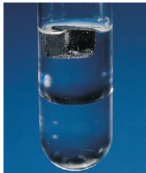
Lithium floating in oil floating on water. Source: © McGraw-Hill Education. Stephen Frisch, photographer
