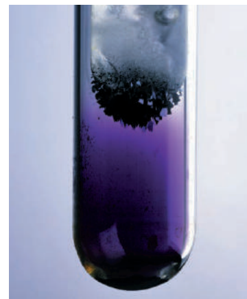
Figure 12.9 Iodine subliming. As the solid sublims, I_2 vapor deposits on a cold surface (water-filled inner test tube).
