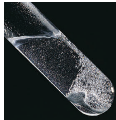
Figure 4.22 The displacement of H 2 from acid by nickel.
