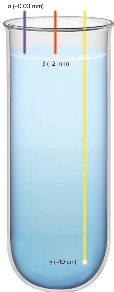
Figure 24.10 Penetrating power of radioactive emissions.
