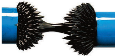
Figure 12.50 The magnetic behavior of a ferrofluid. Nanoparticles of magnetite ( \text{Fe}_3\text{O}_4 ) dispersed in a viscous fluid are suspended between the poles of a magnet.
