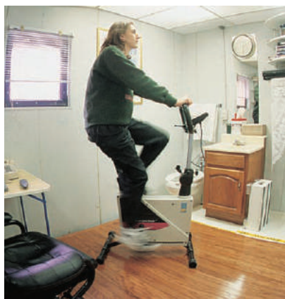
Figure 20.12 A whole-body calorimeter. In this room-sized apparatus, a person exercises while respiratory gases, energy input and output, and other physiological variables are monitored.
