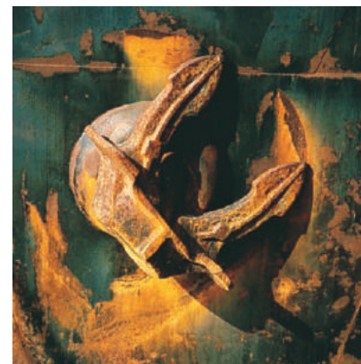
Figure 21.23 Enhanced corrosion at sea. The high ion concentration of seawater enhances the corrosion of iron in hulls and anchors.
