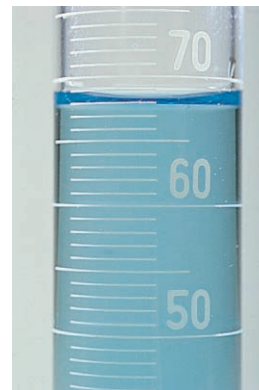
Figure 1.14 Significant figures and measuring devices. The mass measurement (6.8605 g) has more significant figures than the volume measurement (68.2 mL).
